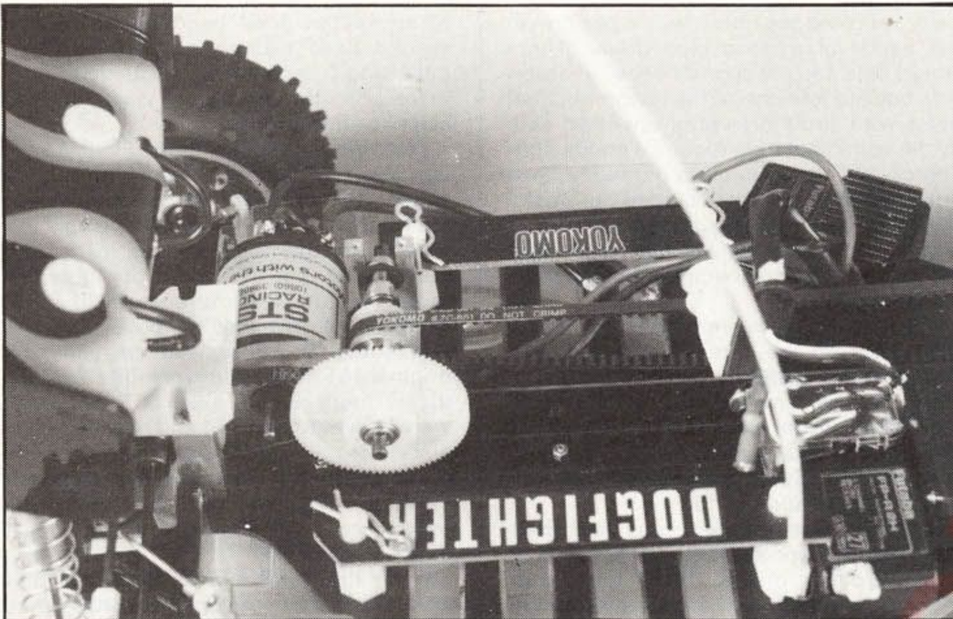
Do not crimp is obvious. The close proximity of the motor to the belt and pulley is shown. The words were rubbed off the belt during testing. Retaining cap on the bulkhead has been removed to show ease of maintenance of component.
