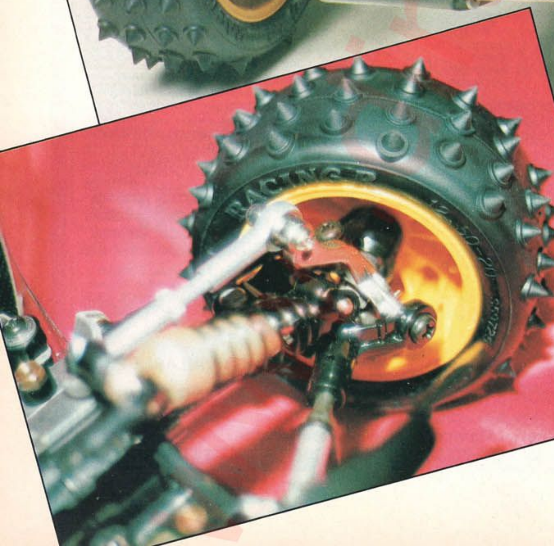
Front upright is beautifully cast in aluminium for extra weight saving.
